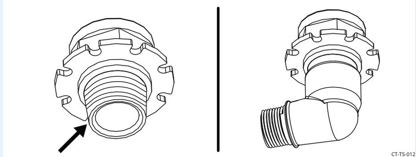
5. **Install** the adapter fittings and elbows onto the water inlets with slip joint pliers. **Tighten** the fittings until the elbows have a slight downward angle.
