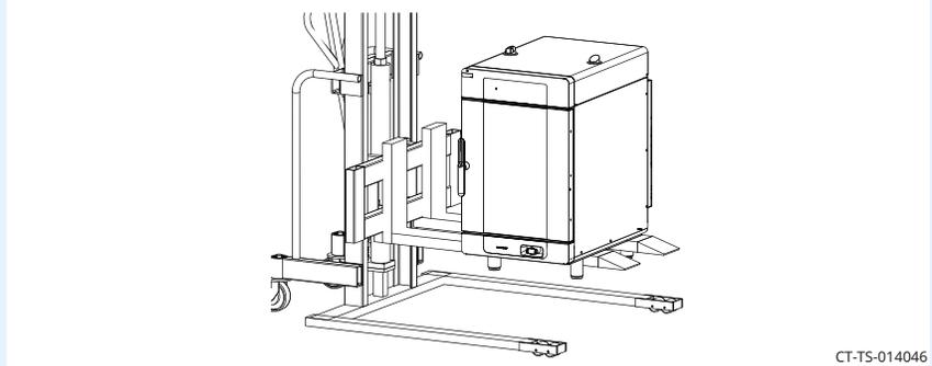
16. **Place** the oven on the stand. Position legs on the outside of the pins.
