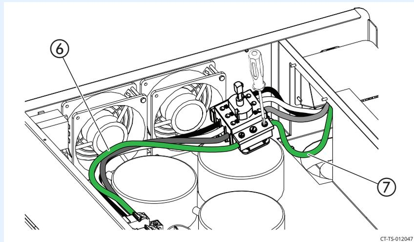
8. **Re-install** the main disconnect switch.
