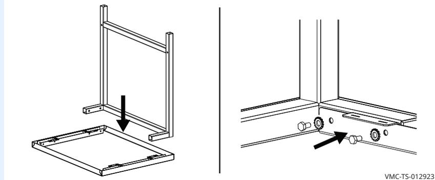
4. **Install** the second leg assembly into the top panel.
