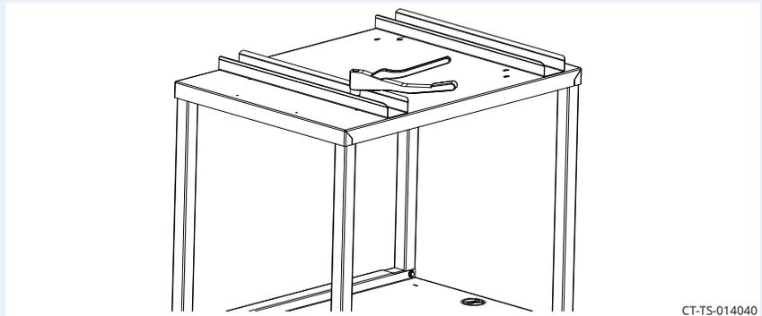
14. **Install** the pins through the channels and the top of the stand. **Secure** the pins with nuts.
