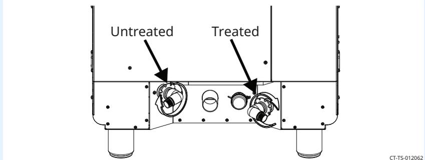
6. **Install** the water hoses onto the elbows.
