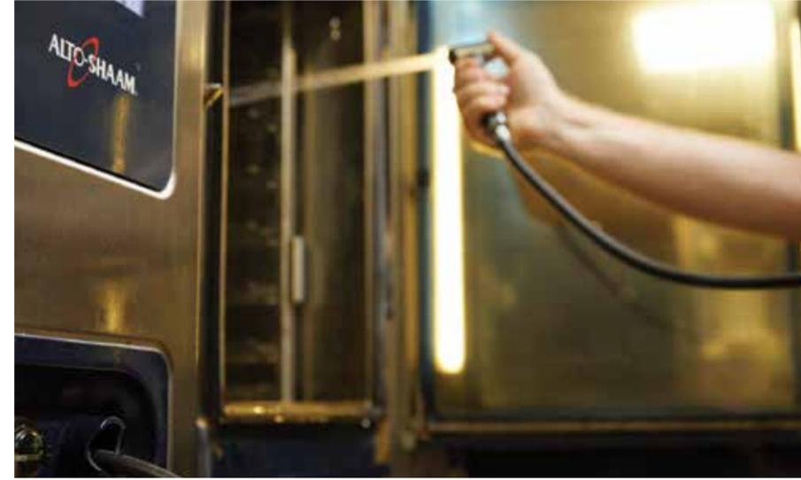
— Front-accessible, retractable rinse hose. PROrinse™ high-efficiency spray head.
